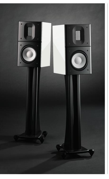
he Raidho Acoustics X1.6 standmount loudspeaker is a rearported design with a 20mm thick aluminium front baffle, housing Raidho's own ribbon tweeter and a 165mm mid-bass unit. The mid-bass driver uses Raidho's own Ceramix technology, which uses a thin aluminium cone bonded with an aluminium-oxide ceramic. Its motor system uses neodymium magnets in a push-pull configuration, providing excellent ventilation and cooling for the titanium voice coil.
